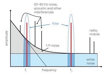
Figure 12. Qualitative noise spectrum of a typical experiment. The measurement frequency should be chosen in a region with small background, avoiding any discrete peaks coming from technical sources. In the example,  $f_2$  will yield better results than  $f_2$  for the same filter bandwidth, since it is located in a clean white noise region above the 1/f noise at low frequencies.
