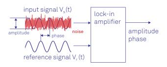
Figure 1. Lock-in amplifiers are capable of measuring the amplitude and the phase of a signal relative to a defined reference signal, even if the signal is entirely buried in noise.
