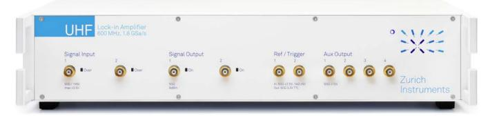
Figure 14. Zurich Instruments UHFLI Lock-in amplifier representing the state of the art of lock-in technology. The 600 MHz signal input bandwidth as well as the 5 MHz demodulation bandwidth make it by far the fastest lock-in amplifier on the market today. In addition, the 19 inch wide instrument integrates the greatest amount of functionality, see Figure 16, while providing the most advanced instrument control software LabOne<sup>®</sup> (see Figure 15).
