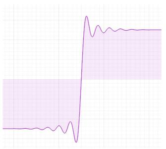
Also called "Sinc" interpolation, this mode preserves the frequency characteristics of the signal. In the time domain though, it can appear that there is over- or under-shoot that is not in fact present in the signal.
