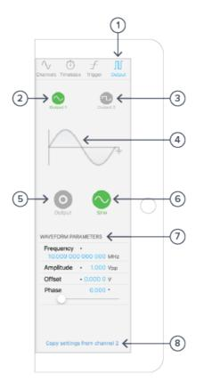
The output pane of the oscilloscope allows for generation of various waveforms on the Moku's output channels.
