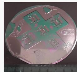
**Figure 2:** Master mold fabricated by UV lithography technique.
