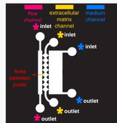
**Figure 1:** Design of LOC device. Left to the right: flow channel, matrix channel and medium channel.
