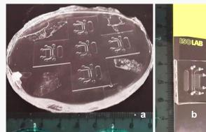
**Figure 3:** a) PDMS LOC image and b) Image of PDMS LOC device after permanent bonding onto glass slide by UV/ozone treatment.
