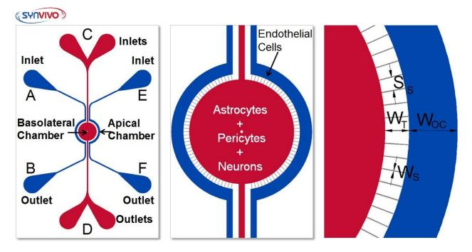
Schematic of the BBB Model Chip. Apical chamber (outer channels) are for culture of vascular (endothelial cells) while basolateral chamber (central chamber) are for culture of brain tissue cells (astrocytes, pericytes, neurons). Porous architecture enables communication between the vascular and tissue cells.
