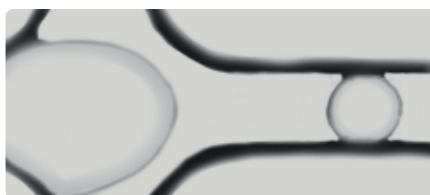
Droplet forming inside the microfluidic chip
