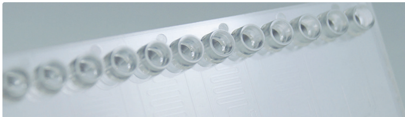
Picture of the topas (COC) microfluidic chip
